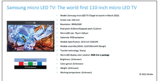
FIGURE 17. Samsung microLED Specifications. Source: Omdia, SAMSUNG—photo taken by Park Ken/Omdia at Consumer Electronics Show (CES) 2020, Las Vegas, NV, January 2020.
