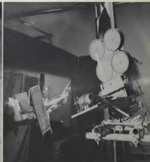
(LEFT) 35mm standard Mitchell camera equipped with pulse drive and selsyn-driven focus cam. This camera is capable of copying over a range from 1-to-1 to infinity, using a 28mm Nikkor lens in bellows mount. (RIGHT) Rigid camera mounts and rigs are readily constructed using 2-inch steel pipe and scaffolding clamps, as shown.
