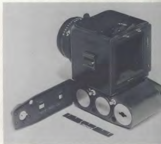
Hasselblad EL/70 Data camera with side-plate removed to show electric drive which advances the film automatically. Special magazines hold up to 200 frames of 70mm black and white film, or 180 frames of color.
