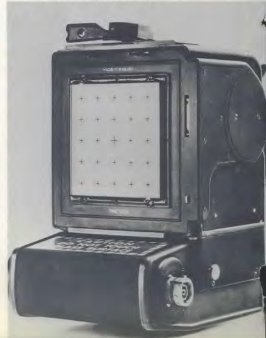
The Reseau grid plate, built into the 500EL Data camera, helps photoanalysts accurately measure subjects photographed.
