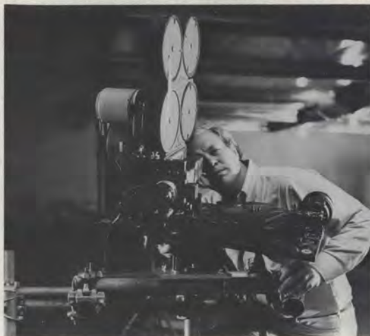
(LEFT) 35mm standard Mitchell camera equipped with pulse drive and selsyn-driven focus cam. This camera is capable of copying over a range from 1-to-1 to infinity, using a 28mm Nikkor lens in bellows mount. (RIGHT) Rigid camera mounts and rigs are readily constructed using 2-inch steel pipe and scaffolding clamps, as shown.
