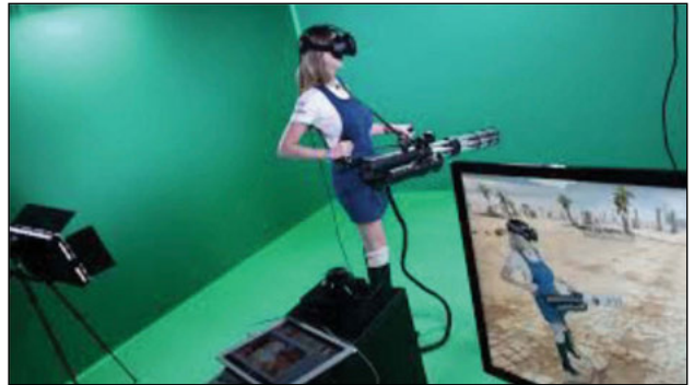
FIGURE 16. MR is the realtime composite from a tracked camera and greenscreen replacement of render content being viewed on the flat panel. The subject is wearing VR goggles that render stereo content of same environment but from her perspective.
