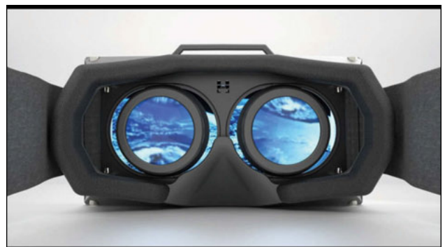
FIGURE 13. VR headset, fully immersed vision of stereo content driven from viewer's perspective.
