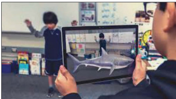
FIGURE 15. AR on mobile tablet, graphics overlay on live video relative to the viewer's perspective.
