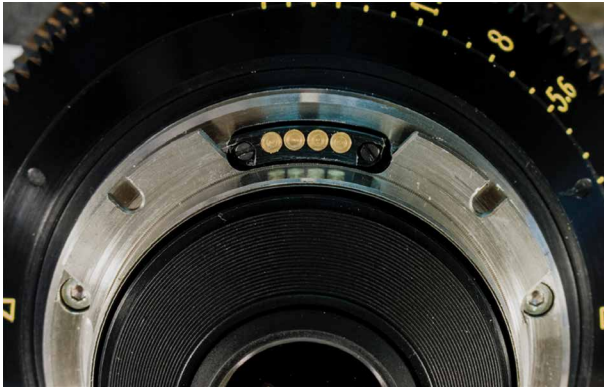
FIGURE 6. PL Mount i-connectors: The four connection points (gold spherical contacts) on the back of a Cook /i smart lens. They are, from left to right, power, data and power, data to the lens and data from the lens. The external interface operates at RS232 levels with standard communication in 8 bit data without parity, 1 stop bit, in ACSII format.
