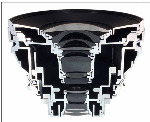
FIGURE 3. A look inside a Zeiss CP2 21mm T2.9 cine lens. This actual lens, sliced on a bandsaw, exposes the intricacies of modern optical and optomechanical design.
